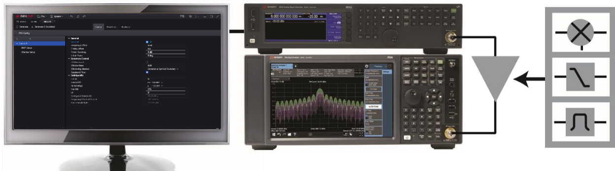
Figure 2. Typical component test configuration using PWSG Desktop with an X-Series signal generator and analyzer.
