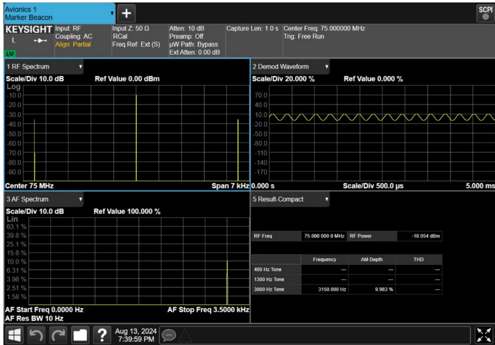
Figure 14. Middle marker beacon signal viewed using a N9040B UXA signal analyzer in the N9092EM0E Avionics measurement application
