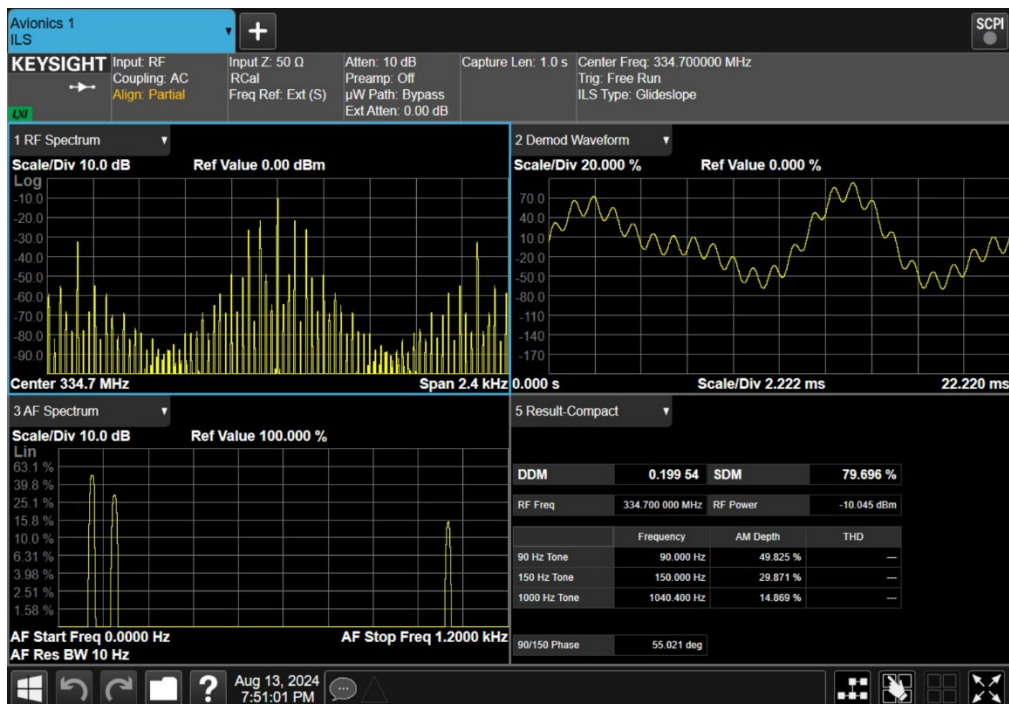
Figure 12. ILS-GS signal viewed using a N9040B UXA signal analyzer in the N9092EM0E Avionics measurement application
