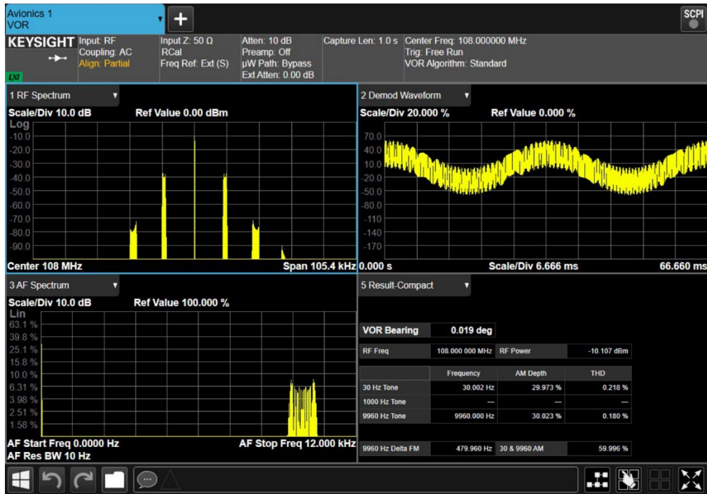
Figure 8. VOR signal viewed using a N9040B UXV signal analyzer in the N9092EM0E Avionics measurement application
