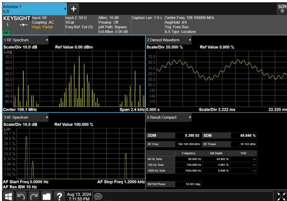
Figure 10. ILS-LOC signal viewed using a N9040B UXA signal analyzer in the N9092EM0E Avionics measurement application
