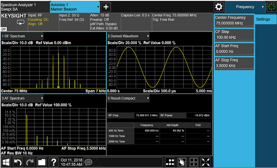
Figure 4. Measurement result for the outer marker at 400 Hz tone, AM depth, frequency and power level of the carrier signal, as well as the spectra of RF and baseband and a demod waveform
