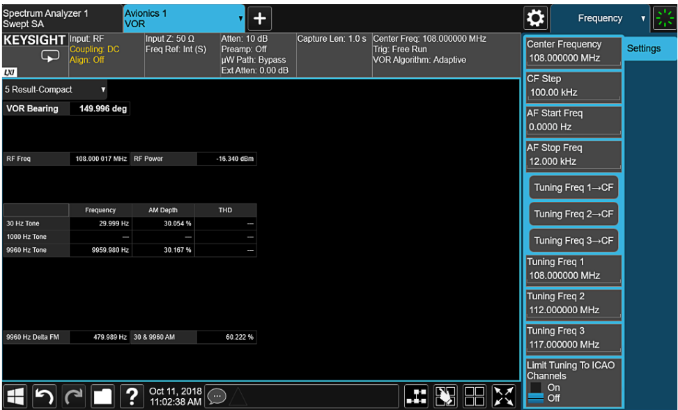
Figure 2. VOR measurement results in numerical form, intuitively showing the key VOR parameters including VOR bearing, frequency and AM depth of the 30-Hz and 9,960-Hz tones, as well as the 1,000-Hz COM/ID tone
