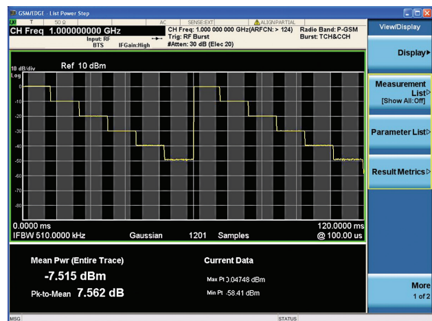
Figure 4. GSM list power step measurement for signal calibration using single acquisition combined measurement mode.
