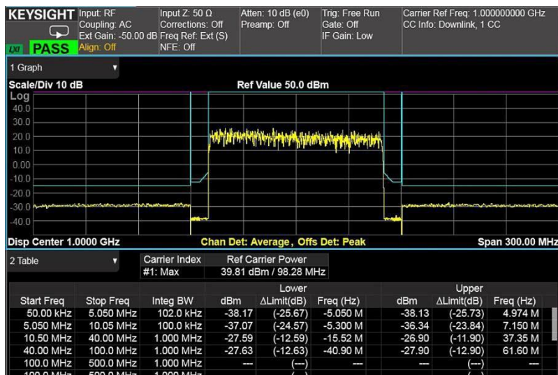
Figure 6. 5G NR Downlink SEM measurement
