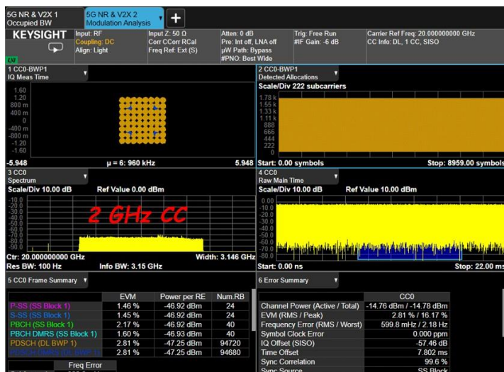
Figure 4. 5G NR Downlink Modulation Analysis measurement with 2000 MHz component carrier
