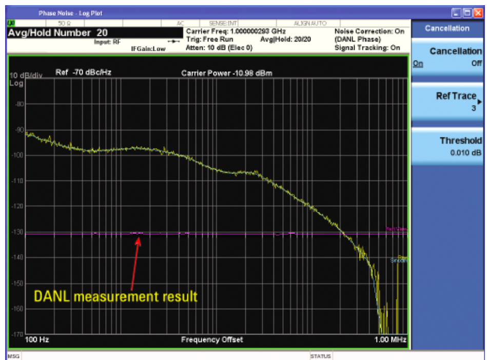
Figure 6. Phase noise plot with subtraction of DANL; the DANL trace is in magenta.
