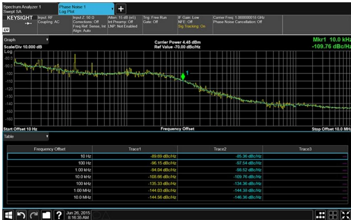
Noise Floor Extensions (NFE) can be used to improve log plot results for far offsets where the DANL floor performance dominates over phase noise performance of the Signal Analyzer. As shown below on a UXA at the 80 MHz offset, the noise floor was lowered by 5 dB when using NFE.
