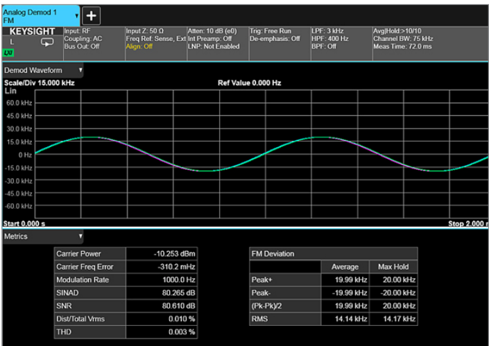
Figure 3. The demod waveform view displays the baseband signal in time domain.
