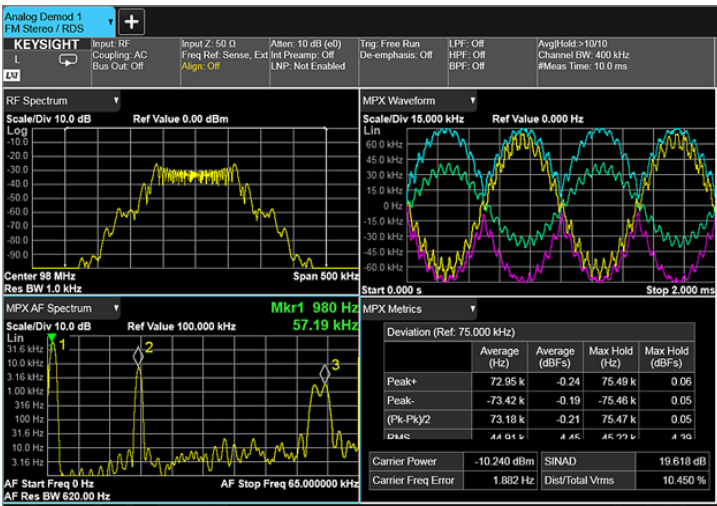
Figure 7. FM stereo MPX view/display with RF spectrum, AF spectrum, demod waveform and demodulation metrics results.
