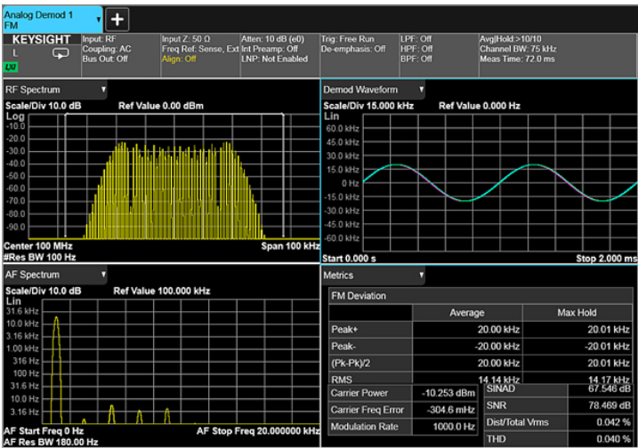
Figure 1. The quad view presents the demodulation metrics results in graph and table simultaneously.
