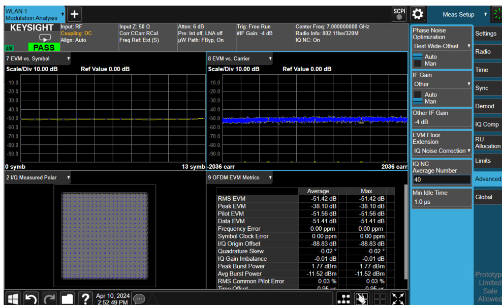
Figure. 802.11be with 320 MHz and MCS13, Frequency: 7 GHz; Power: -10 dBm; IQ-NC on with average 40 Result: EVM performance is improved from -45.5 dB to -51.4 dB
