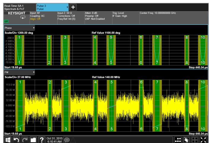
Figure 8. Easily measure pulse linearity and use qualified trigger to select appropriate signal to analyzer.
