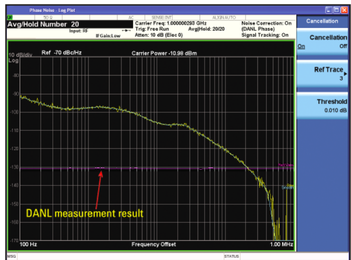
Figure 8. Phase noise plot with subtraction of DANL; the DANL trace is in magenta
