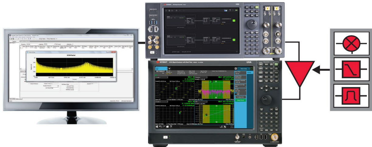
Figure 1. Typical Traveling Wave Tube Amplifier (TWTA) test configuration using Signal Studio for pulse building with M9484C VXG signal generator and N9040B UXA signal analyzer.
