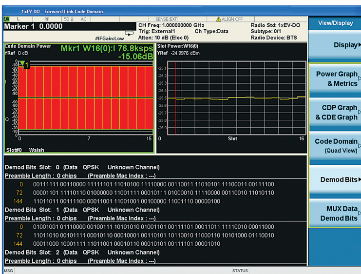
Figure 12. Code Domain for Data Channel—Demod Bits view
