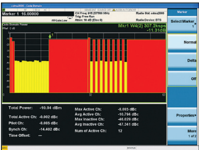
Figure 8. Code domain power measurement marker identifies correct code assignment and power level for active Walsh code W_4^2
