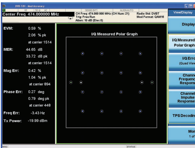
Figure 16. Modulation accuracy measurement with I/Q measured polar graph view
