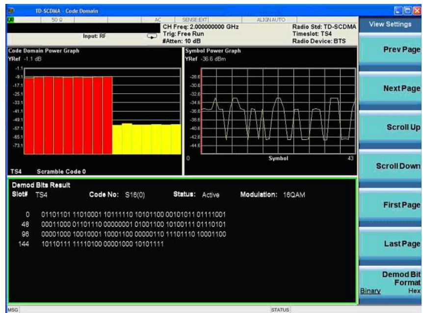
Figure 20. Code domain demodulated bits in binary format; bottom window contains demodulated bits of the selected code channel
