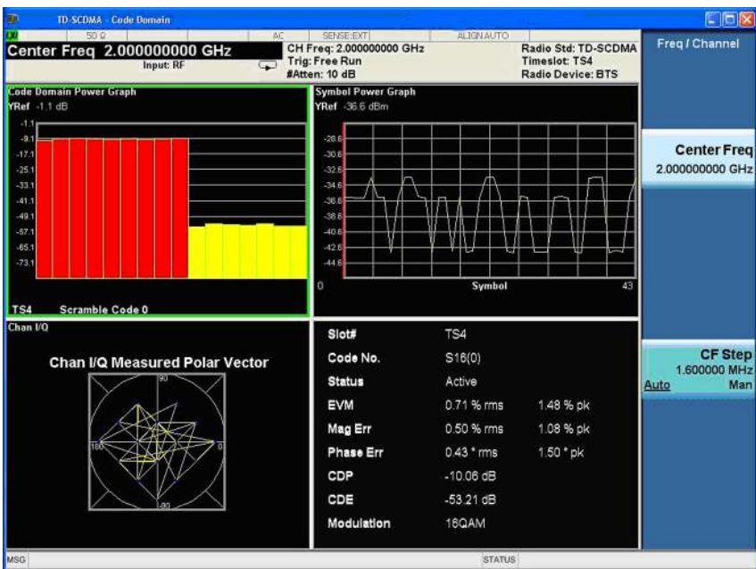
Figure 19. Code domain view showing HSDPA channel with 16QAM modulation
