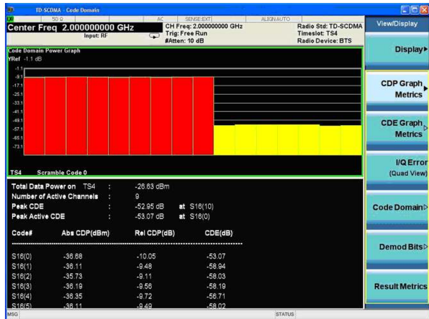
Figure 17. Code domain power (CDP) view shows active and inactive channels, and power metrics of active channels
