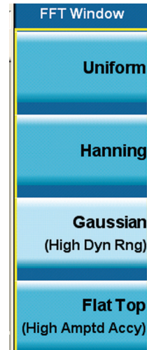
Figure 4. The FFT window filter is applied to each frequency bin, similar to the filter that a spectrum analyzer uses as it sweeps across the frequency span of the measurement; however, with VXA, the filters are applied simultaneously to all frequencies and can be changed.
