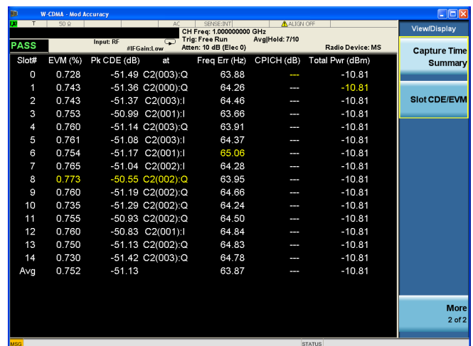
Figure 10. HSPA capture time summary trace showing error metrics for 15 consecutive slots.
