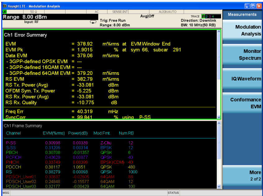
Figure 8. MXG vector signal generator EVM performance of 0.38% at -5 dBm measured using a high-performance PXA signal analyzer with the LTE FDD measurement application. Error summary trace (top): EVM, frequency error, and IQ error results. Frame summary trace (bottom): individual physical signal and channel EVM and power measurement results.
