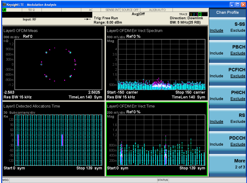
Figure 17. Modulation analysis traces for P-SS, S-SS, and RS only. All other channels were excluded from these measurement results and traces. Any physical channel or signal can be included or excluded in a modulation analysis measurement under {Meas Setup} > {Chan Profile Setup}.
