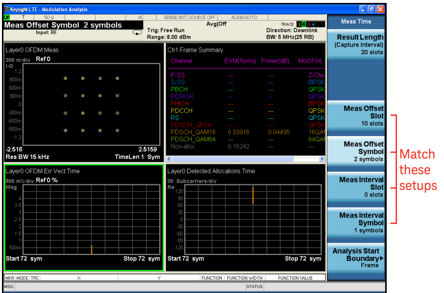
Figure 16. Modulation analysis traces for symbol #2 of slot #10. Note that EVM is reported in the frame summary trace (upper right) only for the 16QAM PDSCH since this is the only channel active during this symbol time. The X-Series signal analyzer LTE measurement applications support demodulation of any user specified slot number and OFDM symbol number within a radio frame. The ability to examine specific slots or symbols individually allows engineers to make all the necessary measurements in order to determine the true root cause of a problem.
