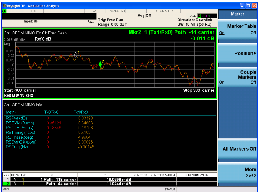
Figure 24. Time offset measurement of 65.1 ns for two simulated Tx antennas measured using an X-Series signal analyzer with the LTE FDD measurement application. The signal is simulated using Signal Studio for 3GPP LTE software and a single MXG vector signal generator. Trace 1 (top): Frequency response of both antenna paths. Trace 2 (bottom): Reference signal power, EVM, time offset, phase, etc., for both transmit paths.
