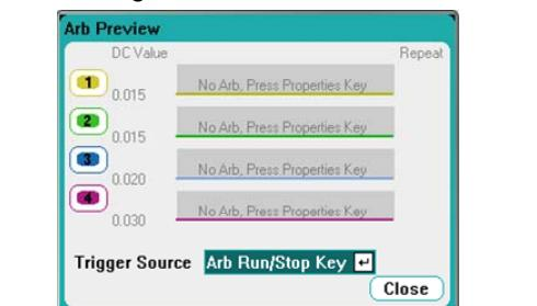
2. Use the navigation keys to select an output. The dark background identifies the selected output. Press the **Enter** key to select the output.
