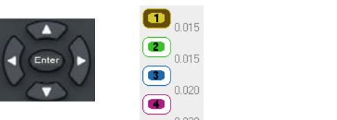
3. Use the navigation keys to select a waveform. Then press **Enter**.
