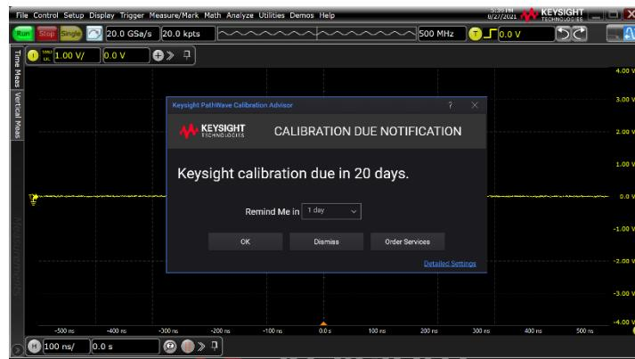
Access your instrument's latest calibration status and information by viewing the electronic calibration label that includes the last calibration date, next calibration due date, and calibration interval. The calibration label eliminates the need to hunt for your instrument's physical calibration sticker.
