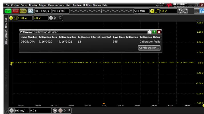
Import your instrument's calibration status document from the main PCA screen. Or use PCA to access calibration certificates and test reports with a link to the online [Keysight Support Portal](#).
