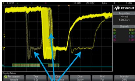
Infrequent glitches and signal jitter captured after 1 second on the 3000 X-Series with standard 1M wfms/s update rate.
