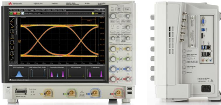
The Keysight Technologies, Inc. S-Series oscilloscope provides bandwidths up to 8 GHz with class-leading signal integrity and analysis. Custom ASICs, including a 40 GSa/s, 10-bit ADC, allow you to see your real signal. Class-leading deep memory and a large suite of analysis tools complement a designed-for-touch user interface and a 15" multi-touch capacitive touch-screen display.
