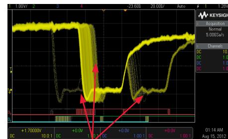
Infrequent glitches and signal jitter captured after 1 second on 3000 X-Series with > 1,000,000 wfms/sec
