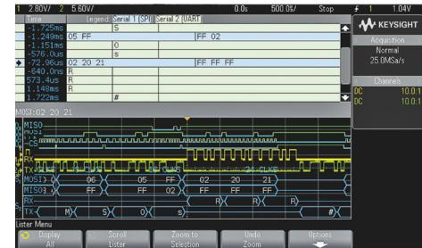
3000 X-Series protocol-aware triggering, decode, search, and navigate for serial buses; hardware-based to maintain fast waveform update rate and capture elusive errors
