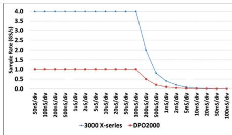
4x the memory allows you to keep sample rates higher on longer time/div settings
