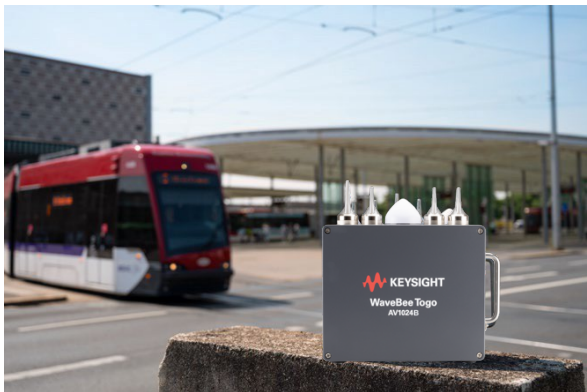
Figure 2. WaveBee Togo generates I2V messages for public transport
