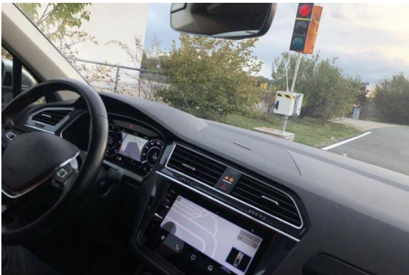
Figure 2. Test drives for checking Road Side Units (RSUs) at traffic signals with WaveBee Plus in the vehicle
