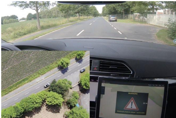
Figure 3. Application for V2X EU Day 1 use case “stationary vehicle” with WaveBee Plus in the vehicle
