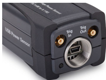
Figure 2. The external trigger input and output ports on the X-Series power sensors.
