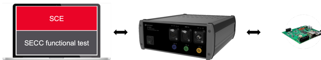
Figure 3. Development tests of SECC with Com Tester and SCE
