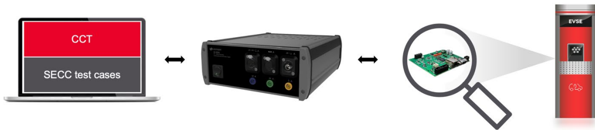
Figure 5. Type approval tests of SECC with Com Tester and CCT
