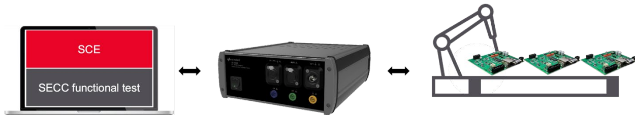
Figure 7. EoL tests of SECC with Com Tester and SCE
