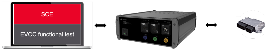
Figure 2. Development tests of EVCC with Com Tester and Smart Charging Emulation Software (SCE)
