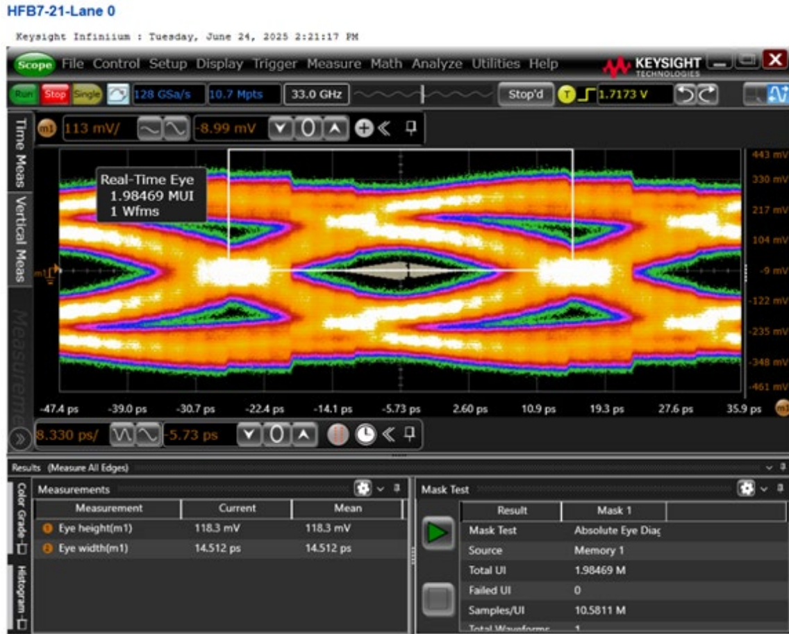
Figure 6. Eye diagram generated by the Infiniium oscilloscope
