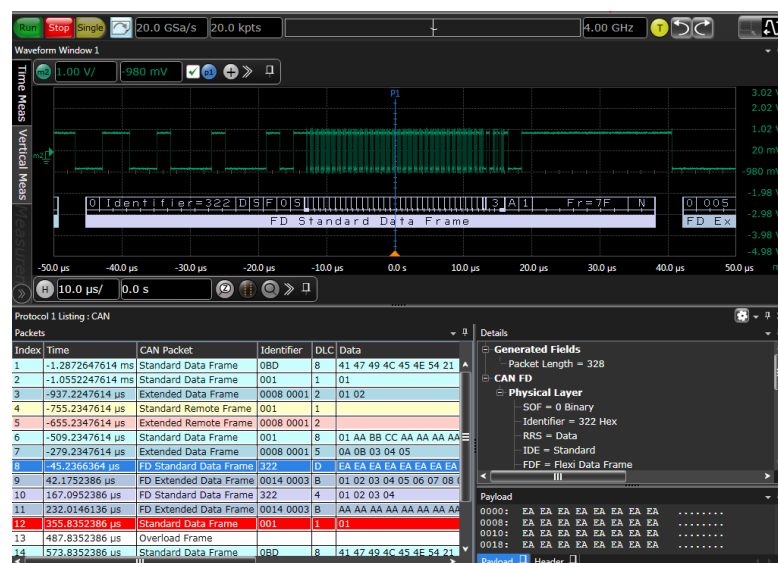
Figure 2. Controller Area Network (CAN) bus decode using Infiniium D9010AUTP software.
