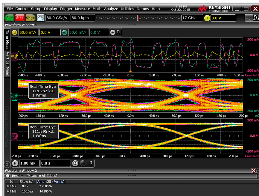
Figure 5. Before and after view of a victim waveform with FEXT using Advanced Signal Integrity software D9010ASIA.
