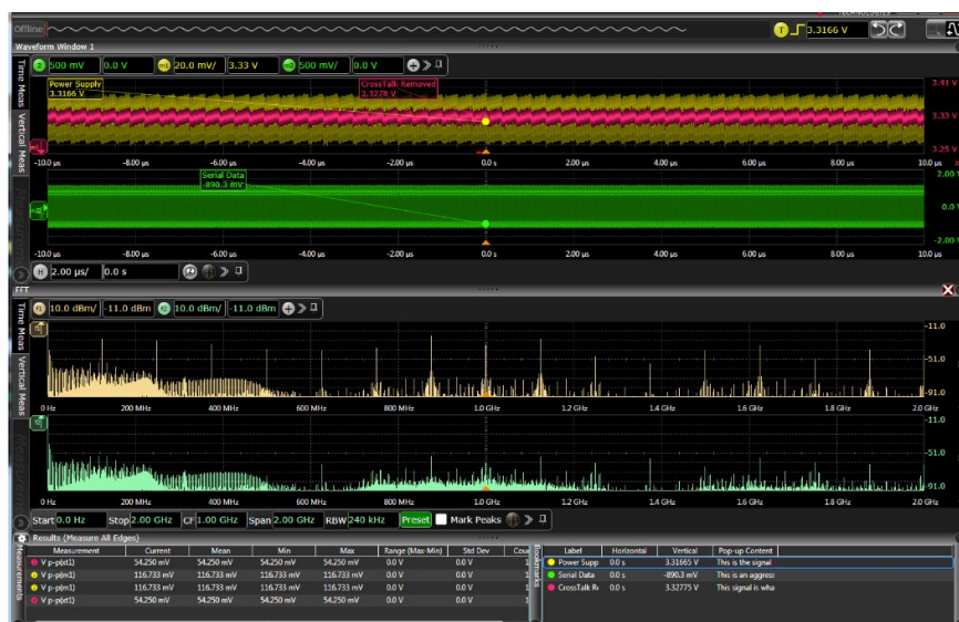
Figure 6. Output from the Power Integrity software application D9010POWA shows a reduction in the noise on a 3.3 V supply after the effects of removing the switching loads.
