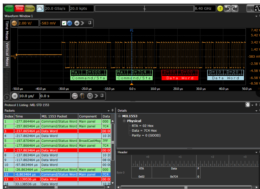
Figure 3. Protocol decoding of MIL-STD-1553 with D9010MILP showing a real-time trace, protocol decoding table, and packet details using a symbolic decode.
