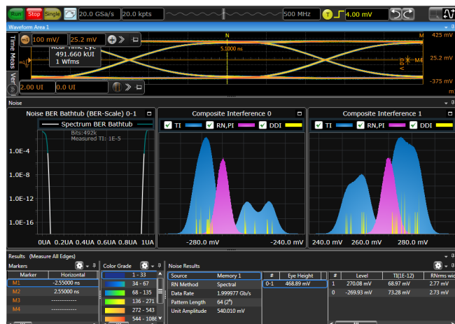
Figure 4. In addition to providing timing jitter separation, EZJIT Complete D9010JITA offers a comprehensive suite of vertical noise separation charts and phase noise measurements.
