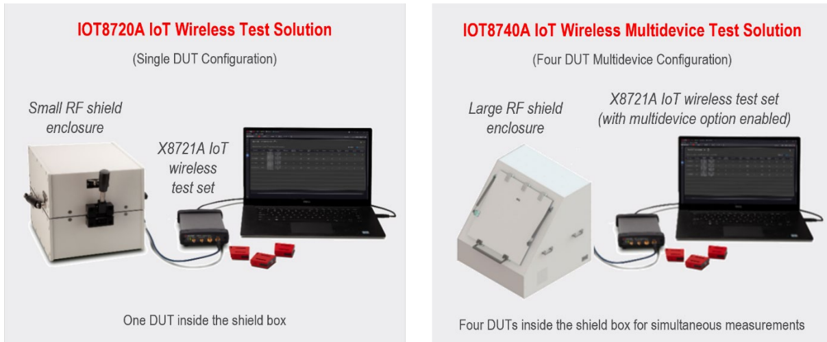
Figure 7. Diagrams showing the single vs multidevice configuration
