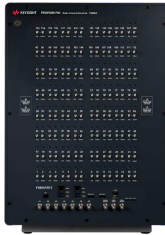
F8800ARF2 RF channel units
