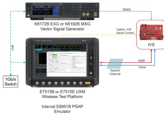
Figure 1. Test Setup 1A: CS eCall - Internal PSAP
