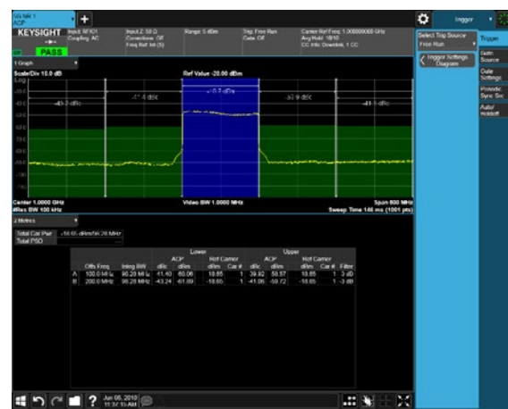
Figure 2. 5G NR adjacent channel power (ACP) results
