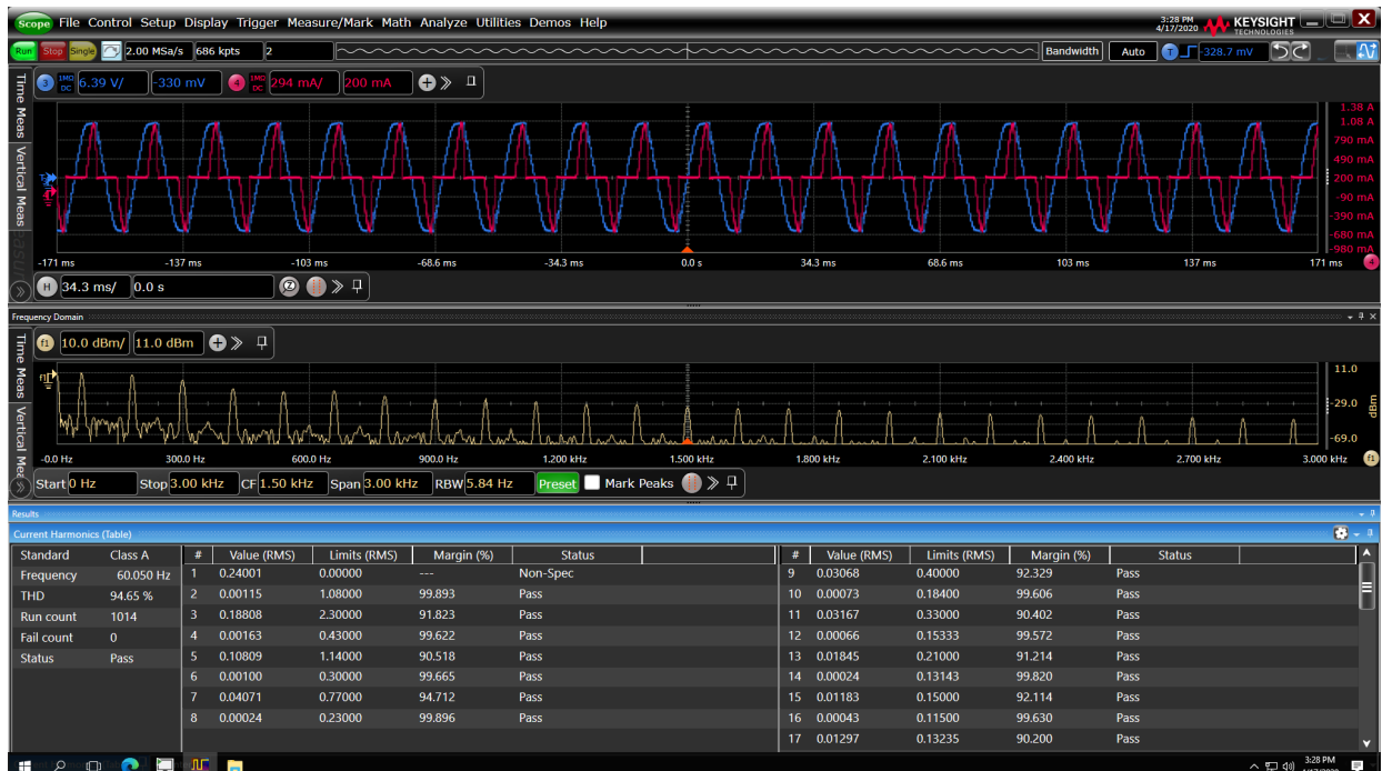
Figure 3. Current harmonics measurement based on IEC 61000-3-2 standards
