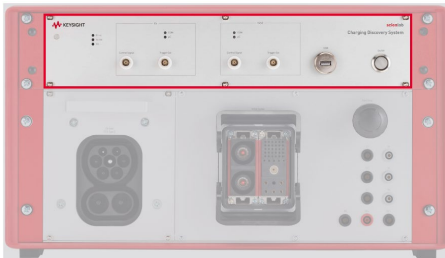
Figure 3. Real-time computer of the Portable CDS
