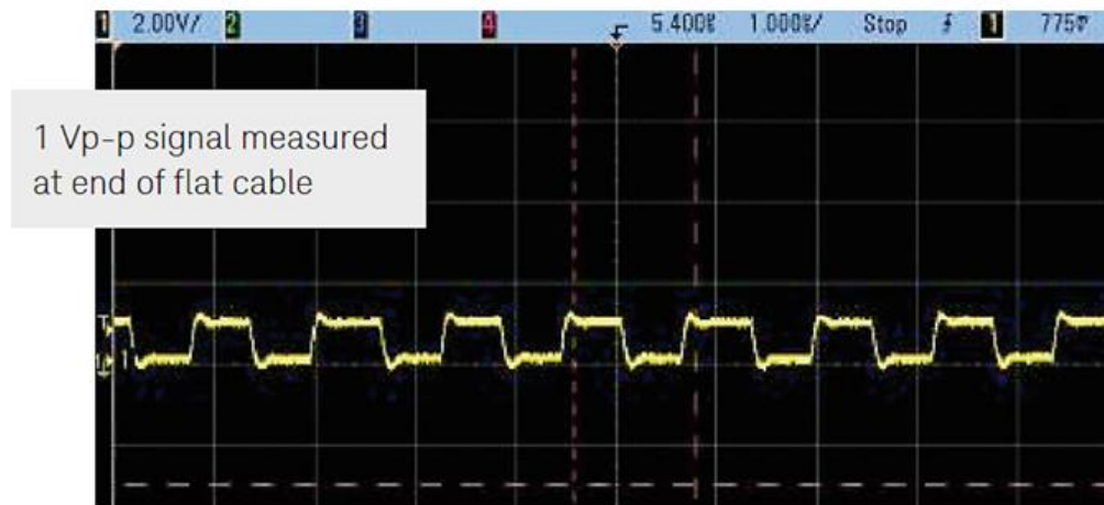
Figure 4. Low signal loss.
