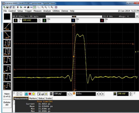
Figure 6. 100 ps pulse with 17 ps risetime.
