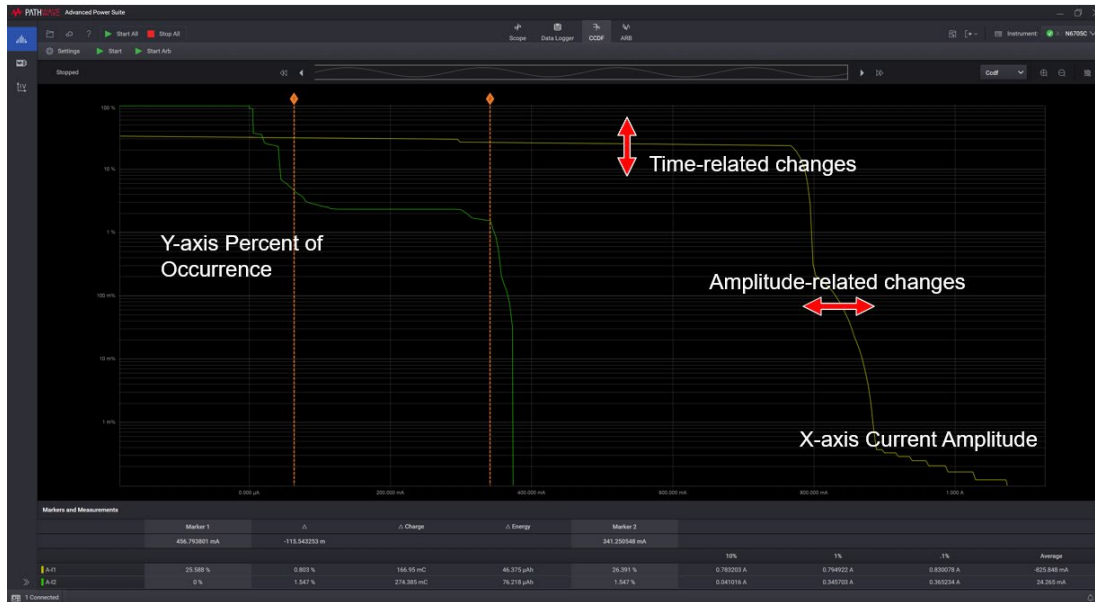
Figure 3. This CCDF measurement reveals the key attributes of standby current in a smartphone.
