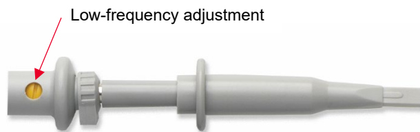
Figure 1. Low-frequency compensation adjustment (for N2889A/90A).
