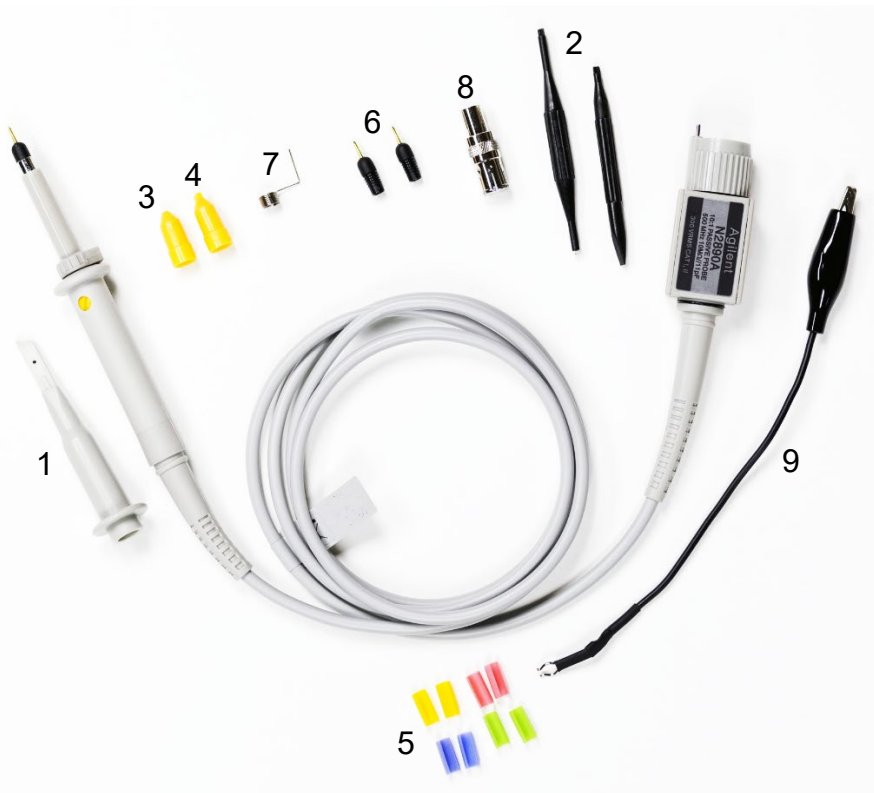
Figure 6. With standard accessories included in the probe
