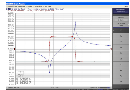
Ceramic resonator measurement with gain-phase series method ( F_r = 400 kHz)
