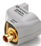
The N5449A high impedance adapter allows connection for probes that require a high impedance scope input such as a high impedance passive probe, 1147B/N2893A current probe, or N2790A differential probe to the Infiniium V, 90000-X/Q Series oscilloscopes. The N5449A provides switchable AC/DC coupling as well as 10:1 and 1:1 attenuation settings. The adapter comes with a N2873A 500 MHz 10:1 passive probe.
