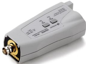
The N5477A sampling oscilloscope adapter makes the Infiniimax III probing system fully compatible with the Infiniium 86100C DCA-J sampling oscilloscope. Previously the DCA-J was limited to 13 GHz of probing, but with the N5477A, the DCA-J now has 30 GHz of probing, increasing its performance and flexibility.
