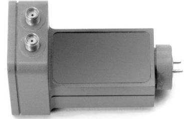
Figure 1. The 11970 Series mixers have separate LO input and IF output ports
