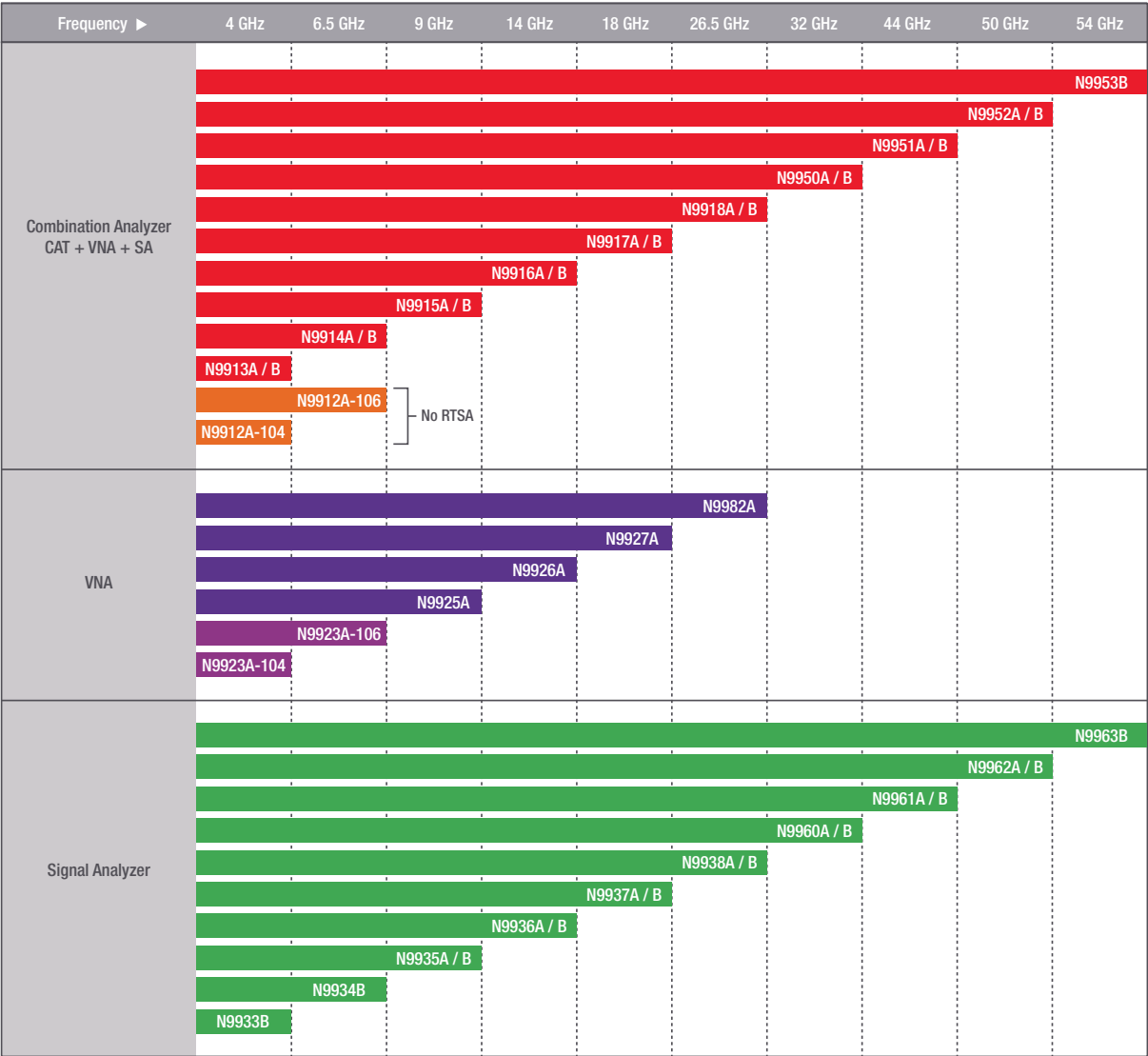
Figure 1. A visual representation of the FieldFox family, base configurations, and frequency coverage
