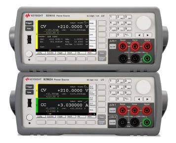
The B2961A / B2962A low-noise power source provides wide bipolar output ranges of 100 nV to 210 V / 10 fA to 10.5 A — and a flexible arbitrary waveform-generation capability. These capabilities make it a suitable voltage or current source for a wide range of material electrical characterization methods, including four-point probe, time of flight, IV, Van der Pauw, and Hall effect measurements.
