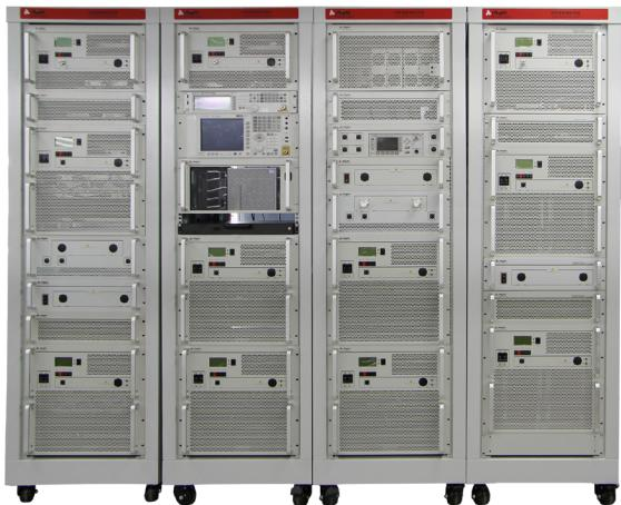
Power tolerance testing is used to verify the performance of components under peak power input signal. It is used to verify the maximum tolerance of a component to withstand heat without degradation and arcing. Power tolerance testing is essential to characterize fully passive components used in telecommunications. These include antennas, duplexers, combiners and cables.
