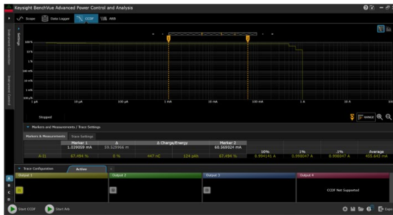
Figure 12. This CCDF measurement reveals the key attributes of standby current in a smartphone.
