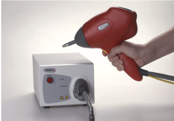
TESEQ Model NSG437 Discharge voltage 200 V-30 kV (IEC61000-4-2-compatible)
