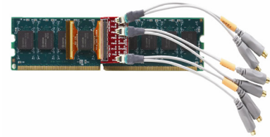
Figure 5: Using an InfiniiMax active differential solder-in probe.
