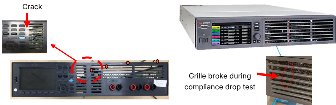
Figure 1. Instrument front housing damage during physical testing
