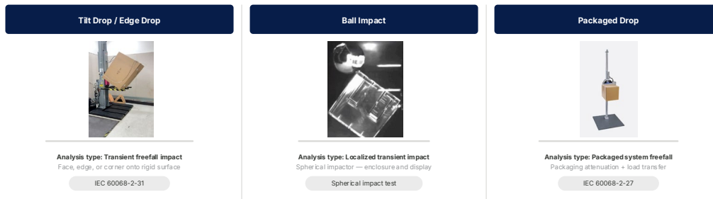
Figure 5. The three common test configurations — tilt/edge drop, ball impact, and packaged drop — cover the primary system-level shock qualification, each implemented as a standardized template within Keysight Multiphysics.
