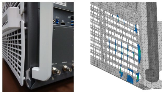
Figure 8. Housing grate deformation after edge drop: physical test result (left) vs. simulation prediction (right). Consistent deformation pattern and magnitude confirm the predictive capability of the model.
